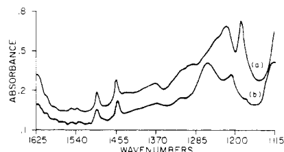
Figure 7. Fourier transform infrared absorption spectra of (a) (±)-mandelic acid [(±)-5] and (b) (±)-mandelic- \alpha -d acid [(±)-8] as 0.5 M solutions in dimethyl- d_6 sulfoxide.
