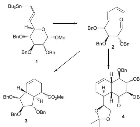
**Figure 1.** Synthesis of polyhydroxylated bicyclic compounds from *D*-gluco-configured allyltin **1**.
