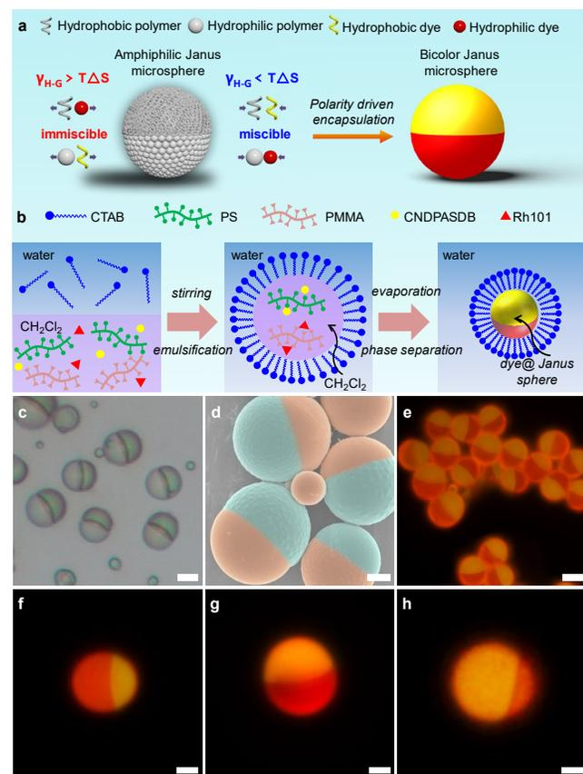
**Figure 1.** (a) Scheme for the design of Janus microspheres with dual-color emission. (b) Illustration for the synthesis of the dual-color Janus microspheres. (c) Optical microscopy images of the Janus microspheres. Scale bar: 5  $\mu$ m. (d) SEM image of the Janus microspheres. Scale bar: 2  $\mu$ m. (e) PL image of the CNDPASDB-Rh101 doped Janus microspheres. Scale bar: 5  $\mu$ m. (f-h) PL images of the CNDPASDB-Rh101 doped Janus microspheres
