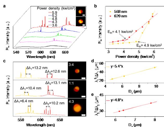
**Figure 2.** (a) PL spectra of a typical CNDPASDB-Rh101 doped Janus microsphere as a function of pump energy. Inset: PL images of the microsphere excited with UV light (top) and focused laser (bottom). Scale bars: 5  $\mu$ m. (b) Power dependent
