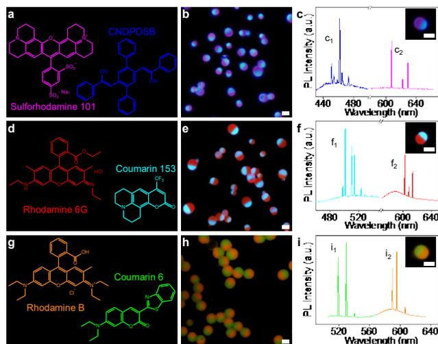
**Figure 4.** Molecular structures of sulforhodamine 101 and CNDPDSB (a); rhodamine 6G and coumarin 153 (d); rhodamine B and coumarin 6 (g). (b, e, h) PL images of the Janus microspheres doped with corresponding dyes. (c, f, i) Normalized lasing spectra of the Janus microspheres shown in the inset. Scale bars: 5  $\mu\text{m}$ .
