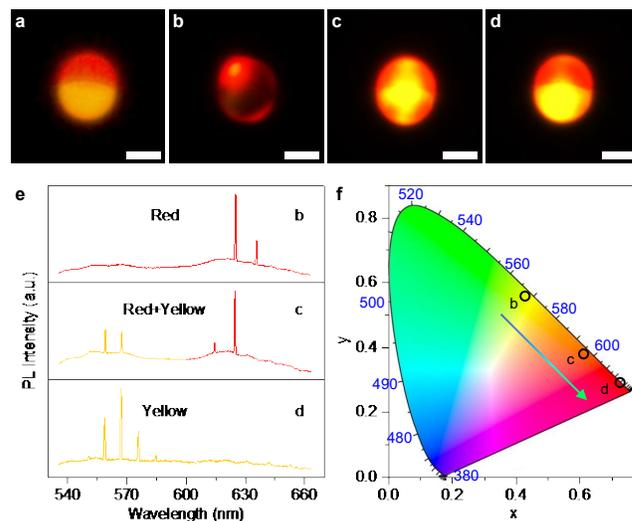
**Figure 3.** (a-d) PL images of the CNDPASDB-Rh101 doped Janus microsphere excited with UV light (a) and focused laser at different positions (b-d). Scale bars: 5  $\mu\text{m}$ . (e) Lasing spectra of the CNDPASDB-Rh101 doped Janus microsphere excited at different positions shown in b-d. (f) Chromaticity of the lasing from b-d
