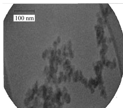
**Figure 1** TEM image of silica chloride nanoparticle.
