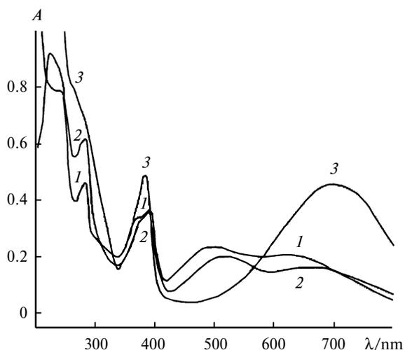
**Fig. 1.** UV-Vis spectra of compound **12** in hexane (**1**) and ethanol (**2**, **3**) before (**2**) and after the addition of NaOH (**3**);  $C = 4 \cdot 10^{-5} \text{ mol L}^{-1}$ .
