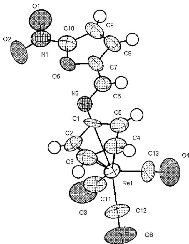
**Fig. 2.** Ortep plot of the asymmetrical unit of **1b**. Relevant bond length (Å): C(1)–N(2) 1.449(16); N(2)–C(6) 1.266(15); C(6)–C(7) 1.439(19); Cp(centroid)–Re(1) 1.961(6) and angles ( $^\circ$ ): N(2)–C(6)–C(7) 122.8(12); C(6)–N(2)–C(5) 120.1(11).
