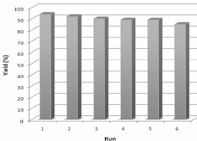
Fig. 3. Investigation of catalyst reusability in the synthesis of TRAMs.
