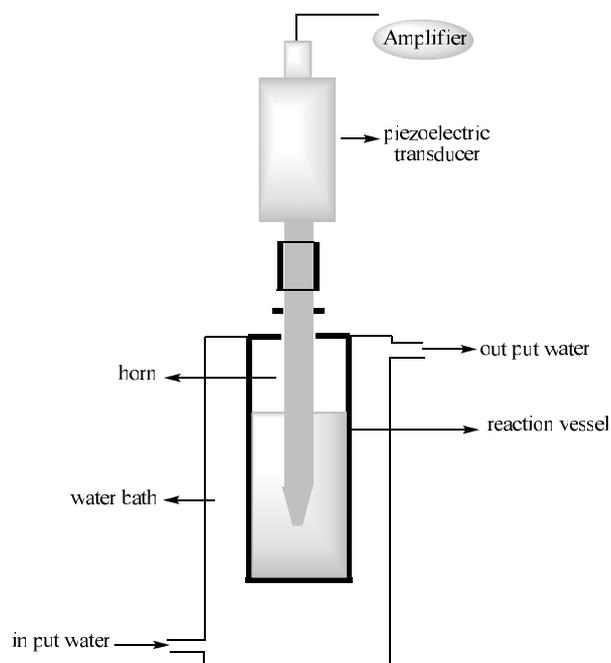
Fig. 1. Ultrasonic experimental set-up.
