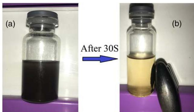
**FIGURE 10** Photographs of aqueous suspension of nano- $\text{Fe}_3\text{O}_4$ @Qs/Ni (II) before (a) and after (b) magnetic capture
