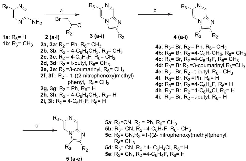
**Scheme 1.** Synthesis of 2-/2, 3-di substituted imidazo[1,2-a]pyrazine (3a–3i, 4a–4i, 5a–5e). Reagents and conditions: (a) acyl bromide, NaHCO<sub>3</sub>, EtOH, reflux; (b) N-bromo-succinimide, EtOH, RT; and (c) CuCN, DMF, reflux.
