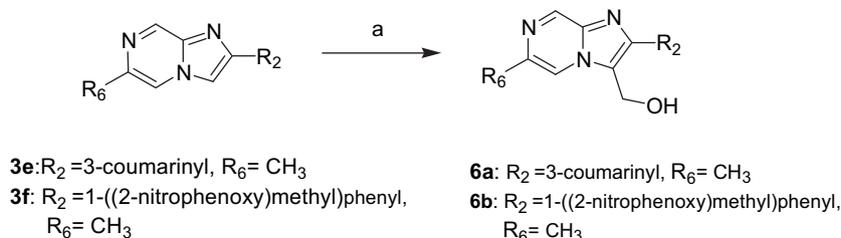
**Scheme 2.** Synthesis of 3-hydroxymethyl-2-substituted imidazo[1,2-a]pyrazine. Reagents and conditions: (a) formaldehyde, acetic acid, acetic anhydride, 60 °C.
