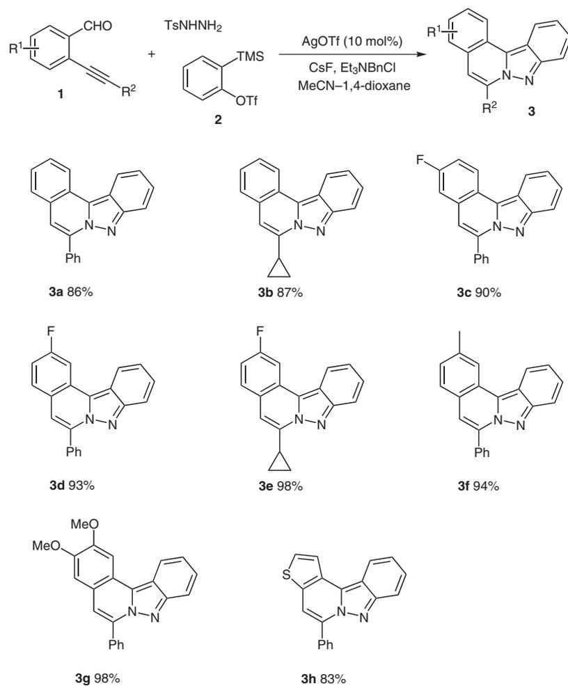
**Scheme 2** Synthesis of *H*-pyrazolo[5,1-*a*]isoquinolines through a three-component reaction of 2-alkynylbenzaldehyde, tosylhydrazine, and benzyne
