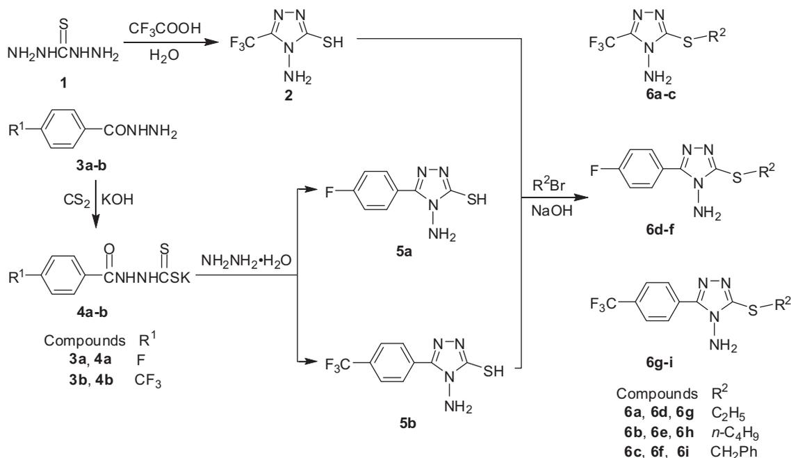
**Scheme 1.** Synthesis of some 3,5-disubstituted-4H-1,2,4-triazol-4-amines.
