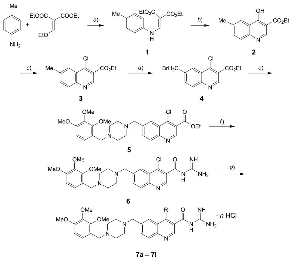
a) 110°, N<sub>2</sub>. b) Ph<sub>2</sub>O, 250°, N<sub>2</sub>. c) POCl<sub>3</sub>, reflux. d) *N*-Bromosuccinimide (NBS), CCl<sub>4</sub>, benzoyl peroxide, reflux. e) Trimetazidine, MeCN, K<sub>2</sub>CO<sub>3</sub>, r.t. f) Guanidine, *i*-PrOH, r.t. g) 1. Alkylamine or substituted phenylamine, *i*-PrOH, K<sub>2</sub>CO<sub>3</sub>, reflux, 2. sat. HCl (g) in anh. AcOEt (except for **7d** and **7h**).
