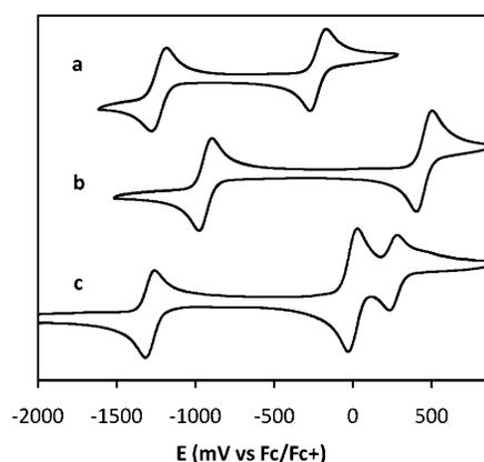
**Figure 1.** Cyclic voltammograms of (a) **1a**, (b) **2a**, and (c) **2b**. The redox event centered at 0 mV in (c) corresponds to the ferrocene/ferrocenium redox couple (ferrocene added as an internal reference). All CVs performed in MeCN solution at scan rates of 100 mV/s with 0.1 M Bu<sub>4</sub>NBF<sub>4</sub> electrolyte.
