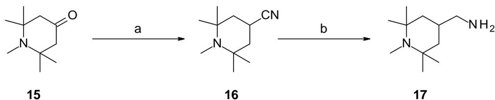
**Scheme 5.** Reagents and conditions: (a) TosMIC, <sup>t</sup>BuOK, DME, rt, 2 h; (b) LAH, THF, 0 °C, 3 h.
