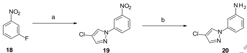
**Scheme 6.** Reagents and conditions: (a) 4-Cl-1H-pyrazole,  $K_2CO_3$ , DMI, 130 °C, 16 h; (b)  $SnCl_2 \cdot 2H_2O$ , EtOH, reflux, 6 h.
