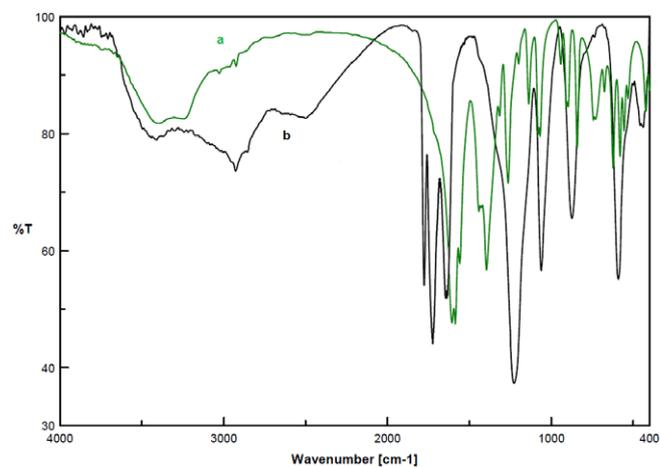
FIGURE 1 FT-IR spectra of (a) trisodium citrate and (b) citrate trisulfonic acid
