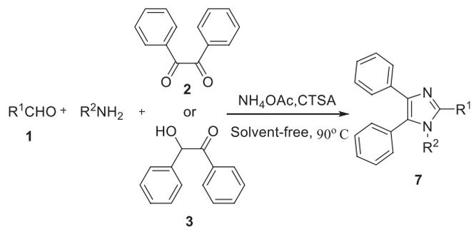
SCHEME 2 Synthesis of 1,2,4,5-tetrasubstituted imidazoles
