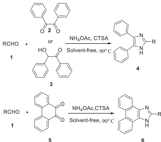
SCHEME 1 Synthesis of 2,4,5-trisubstituted imidazoles
