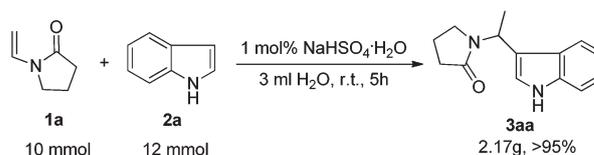
**Scheme 2** A large-scaled reaction under neat conditions.
