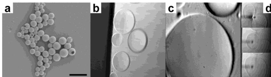
**Figure 2.** (a) Scanning electron micrograph of PS-PIAT vesicles, formed by the injection method, after 2 days in dispersion; the scale bar represents 5  $\mu\text{m}$ . (b, c) Optical micrographs of electroformed giant vesicles of PS-PIAT; the image width corresponds to 60  $\mu\text{m}$ . (d) Two giant vesicles fuse into one vesicle with the help of a micropipet. The width of the optical micrographs amounts to 80  $\mu\text{m}$ .
