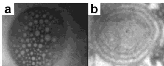
**Figure 3.** Fluorescence micrographs of fluorescein-labeled dextran inside electroformed giant vesicles of PS-PIAT. (a) Multicompartmental giant vesicle; the width of the image corresponds to 80  $\mu\text{m}$ . (b) Multilamellar giant vesicle; the width of the image corresponds to 45  $\mu\text{m}$ .
