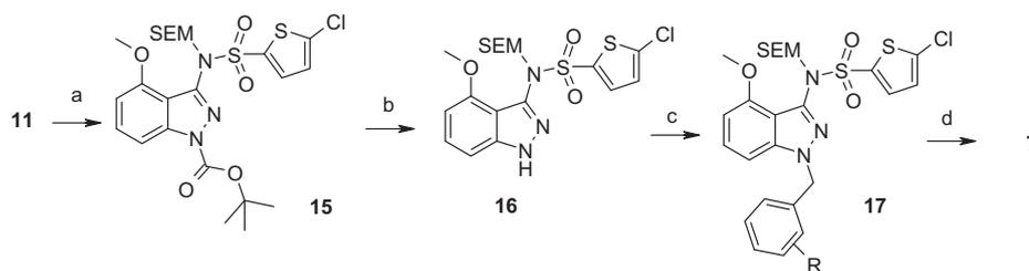
**Scheme 2.** Reagents and conditions: (a) SEM-Cl, DIPEA, DCM, 100%; (b)  $\text{Na}_2\text{CO}_3$ ,  $\text{H}_2\text{O}$ , DMF, 85 °C, 74%; (c)  $\text{ArCH}_2\text{Br}$ ,  $\text{K}_2\text{CO}_3$ , DMF, 44–88%; (d)  $^t\text{Bu}_4\text{NF}$ , THF, 90–95%.
