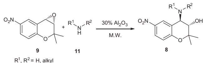
Scheme 3. Microwave assisted aminolysis in the presence of neutral alumina.
