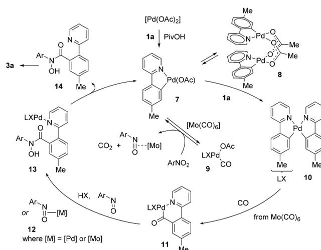
**Scheme 3.** Possible catalytic cycle for Pd-catalyzed aminocarbonylation.
