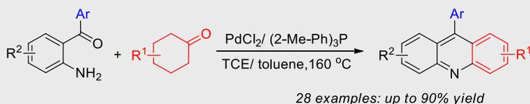
An efficient strategy for 9-aryl-substituted acridine synthesis from cyclohexanones and 2-aminobenzophenones under palladium-catalyzed conditions has been developed. Using molecular oxygen as the green oxidant, various cyclohexanones were acted as aryl source to construct the nitrogen-containing heterocycles via condensation/cyclization/tautomerization sequence.
