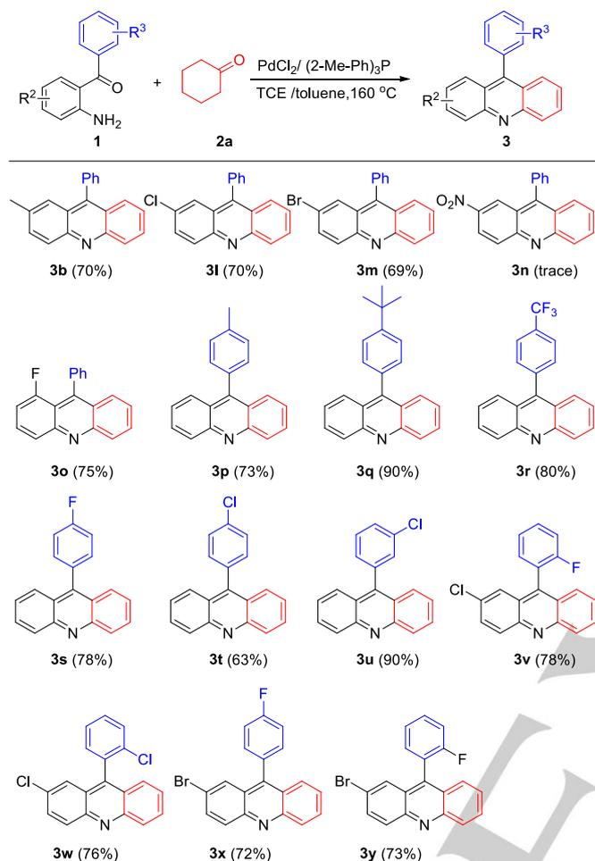
[a] Conditions : **1** (0.4 mmol), **2a** (0.2 mmol), PdCl<sub>2</sub> (10 mol%), tri-*ortho*-tolylphosphine (10 mol%), 1,1,2,2-tetrachloroethane (TCE, 0.6 mL), toluene (0.2 mL), 160 °C, 24 h, under oxygen atmosphere. [b] Isolated yield based on **2a**.
