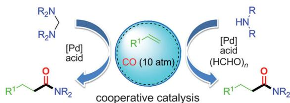
**Back to basics:** The basicity of aliphatic amines precludes their use in the palladium-catalyzed hydroaminocarbonylation. This issue was overcome by using aminals as surrogates of aliphatic amines. A cooperative catalytic system
