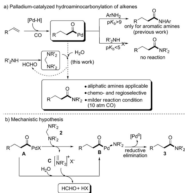
**Scheme 1.** Proposed palladium-catalyzed hydroaminocarbonylation of alkenes with aminals.
