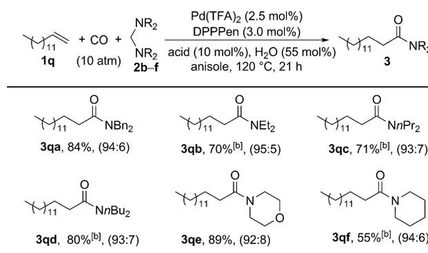
[a] General conditions: **1 q** (0.8 mmol), **2** (0.2 mmol), CO (10 atm), Pd(TFA)<sub>2</sub> (0.01 mmol), DPPPen (0.012 mmol), NH<sub>2</sub>CH<sub>2</sub>CO<sub>2</sub>Me·HCl (0.04 mmol), and H<sub>2</sub>O (0.22 mmol) in anisole (1.0 mL) at 120 °C for 21 h. Yield of isolated linear product based on amino moiety; the l/b ratios within parentheses were determined by GC and GC-MS analysis. [b] Acid (0.2 mmol).
