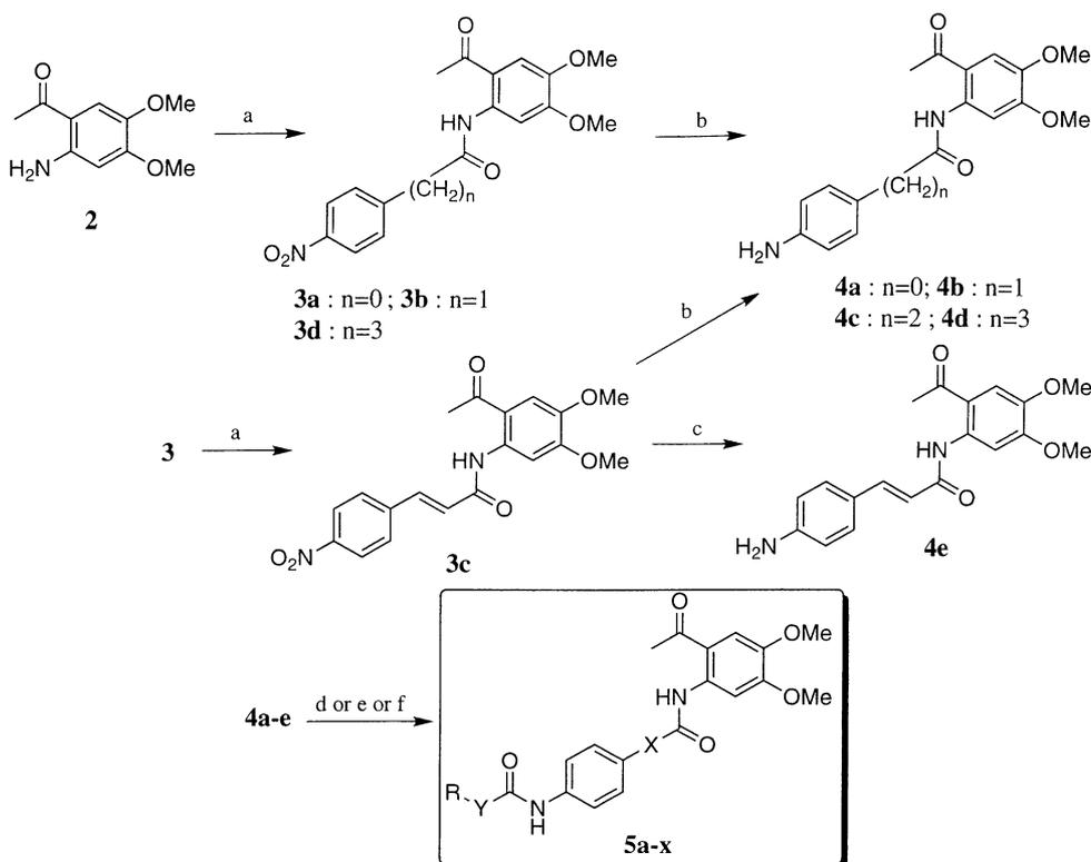
Scheme 1. Synthesis of compounds **5a–x**. Reagents and conditions: (a) (4-NO<sub>2</sub>-Ph)-X-COCl, Et<sub>3</sub>N/CH<sub>2</sub>Cl<sub>2</sub>; (b) H<sub>2</sub>, 5% Pd/C, EtOH; (c) Fe, AcOH; (d) RNCO, DMAP/THF; (e) Ph-Y-COCl, Et<sub>3</sub>N/CH<sub>2</sub>Cl<sub>2</sub>; (f) PhOH, CDI/THF then DBU.
