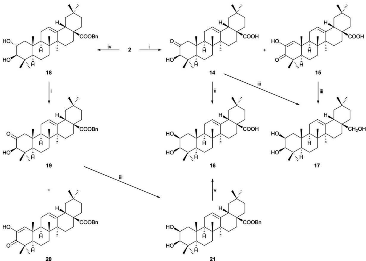
**Scheme 3.** (i) PCC/DCM. (ii) NaBH<sub>4</sub>/i-PrOH. (iii) LiAlH<sub>4</sub>/THF. (iv) BnCl/K<sub>2</sub>CO<sub>3</sub>/DMF. (v) H<sub>2</sub>/Pd/DCM.
