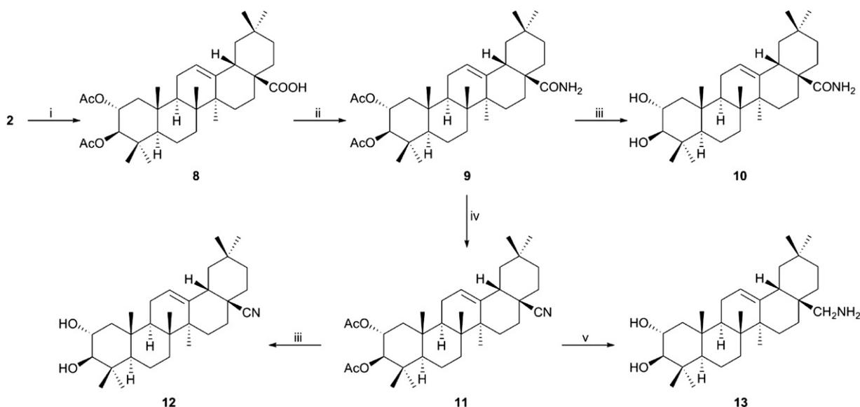
**Scheme 2.** (i) Ac<sub>2</sub>O/Py. (ii) 1) SOCl<sub>2</sub>/DCM, 2) MeOH/NH<sub>3</sub> (1:1). (iii) KOH/MeOH (1:10). (iv) SOCl<sub>2</sub>/DCM. (v) LiAlH<sub>4</sub>/THF.
