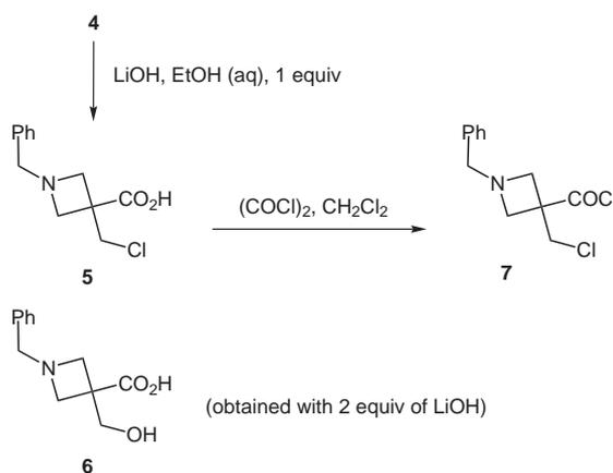
**Scheme 3** Hydrolysis of ester **4** and preparation of acid chloride **7**
