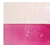
Fig. 3 Compound **5a** in methyl stearate (lower cold, upper warm).
