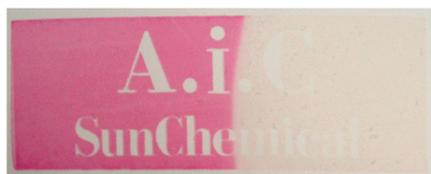
Fig. 4 Screen printed label containing **5a** (LHS cold, RHS warm).
