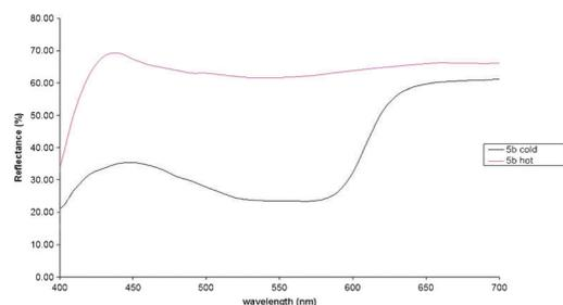
Fig. 6 Reflectance spectra of **5b** in methyl stearate containing bisphenol A at 20 °C and 50 °C.
