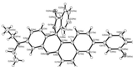
Fig. 1 X-ray crystal structure of **5a** with thermal ellipsoids scaled at the 50% probability level.
