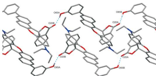
Fig. 2 Stick view of compound **5a** showing the hydrogen-bonded chains of alternating A and B molecules.Table 1 Bond lengths and angles for intermolecular H-bonds between donor (D) and acceptor (A) groups for chains of **5a**
