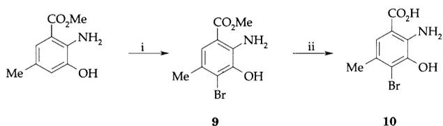
**Figure 3.** i)  $\text{Br}_2/\text{HOAc}$ , ii)  $\text{KOH}/\text{EtOH}$ .
