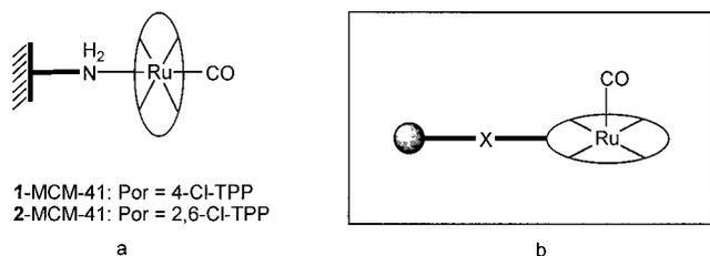
**Figure 1.** Schematic structures of ruthenium porphyrins (a) coordinatively grafted onto surface modified MCM-41 and (b) covalently attached to a solid support. 4-Cl-TPP = *meso*-tetrakis(4-chlorophenyl)-porphyrinato dianion; 2,6-Cl-TPP = *meso*-tetrakis(2,6-dichlorophenyl)-porphyrinato dianion.
