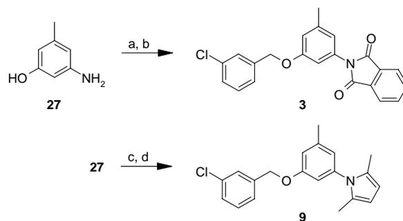
**Scheme 1.** Reagents and conditions: (a) phthalic anhydride, acetic acid, 1.5 h reflux; (b) 3-chlorobenzyl chloride,  $CS_2CO_3$ , DMF, 1.5 h 100 °C; (c) NaH, DMF, 45 min rt, then 3-chlorobenzyl bromide, 12 h rt; (d) acetylacetone,  $pTsOH \cdot H_2O$ , toluene, 1.5 h reflux (water trap).
