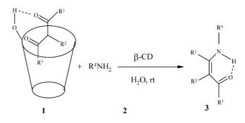
The results are summarized in Table 1. The reactions were completed at room temperature within 5-90 min. The products were obtained in excellent yields and chemo-selectivity to afford *Z*- $\beta$ -enaminones, confirmed by <sup>1</sup>H NMR spectrum of the crude products ( $\delta$  = 7.5-12.8 for NH).
