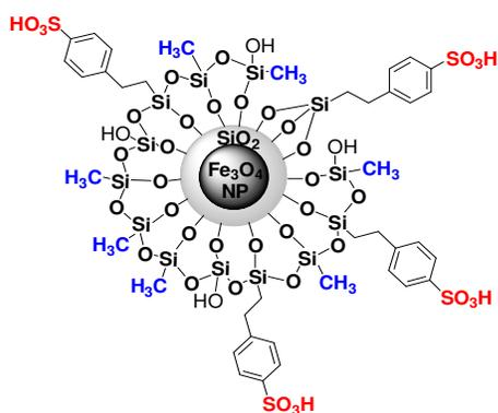
**Figure 1.** The hydrophobic magnetic solid sulfonic acid catalyst,  $\text{Fe}_3\text{O}_4@SiO_2@Me\&Et-PhSO_3H$ .
