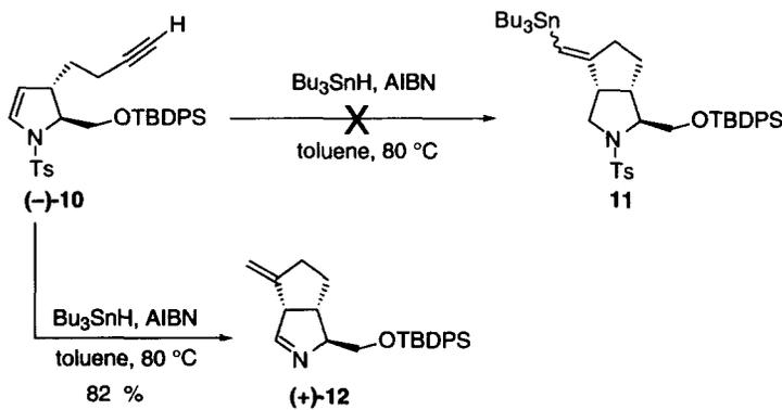
The obtainment of (+)-**12** can be explained by the attack of the tri-*n*-butylstannyl radical onto the tosyl group<sup>34</sup> of (–)-**10**. This implies the formation of the ene-aminy radical  $13 \leftrightarrow 13'$ . A 5-*exo*-dig cyclization<sup>35</sup> takes place and produces radical intermediate **14** which, after reduction, affords the observed bicyclic imine (+)-**12** (Scheme 7).
