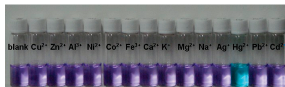
Figure 1. Color changes upon addition of different metal ions (10 equiv) to SQ-1 (2 \mu\text{M} ) in AcOH– \text{H}_2\text{O} (40:60, v/v) solution.
