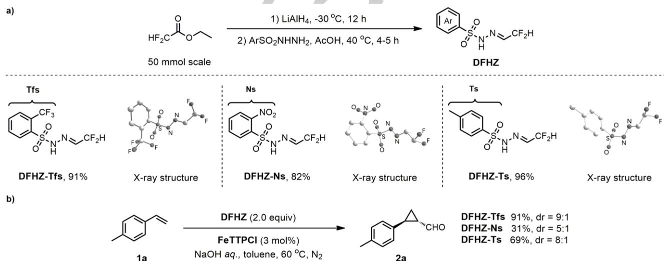
**Scheme 1.** a) Preparation of difluoroacetaldehyde *N*-sulfonylhydrazones (DFHZ). b) Fe-catalyzed cyclopropanation with *p*-methylstyrene.
