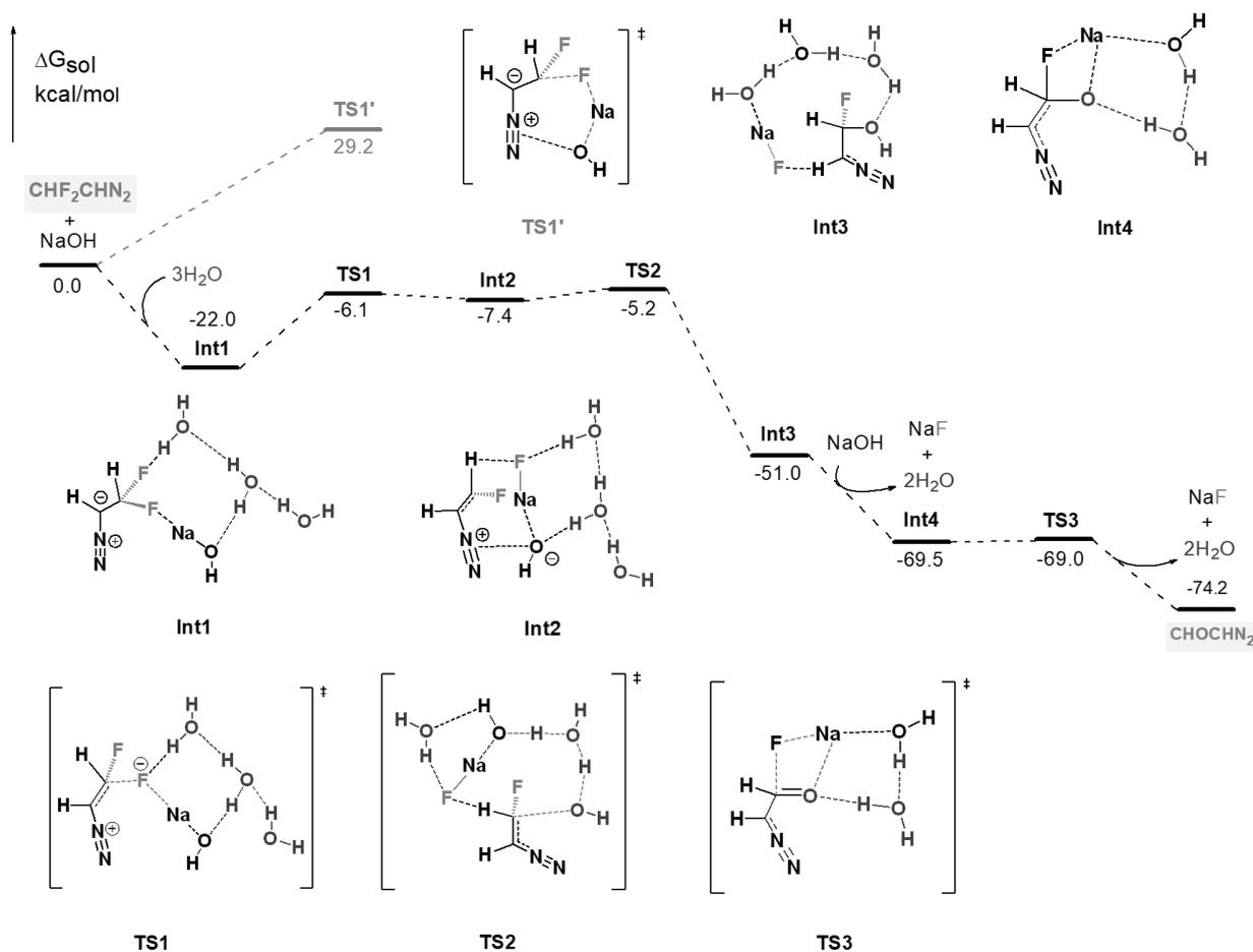
Figure 2. Free energy profiles of the conversion of  $\text{CF}_2\text{HCHN}_2$  into  $\text{CHOCHN}_2$ .
