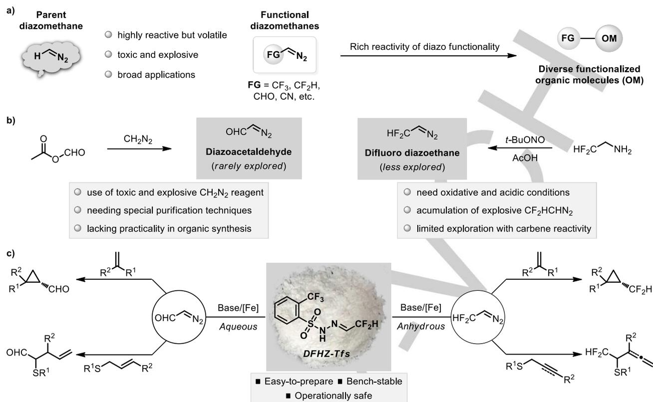
**Figure 1.** a) The functionalized diazomethane strategy for introducing functional groups into organic molecules by virtue of the reactivity of diazo functionality. b) Previous approaches to the generation of two important volatile functionalized diazomethanes. c) Our strategy for the in situ safe and divergent generation and reactions of diazoacetaldehyde and difluorodiazomethane from DFHZ-Tfs.
