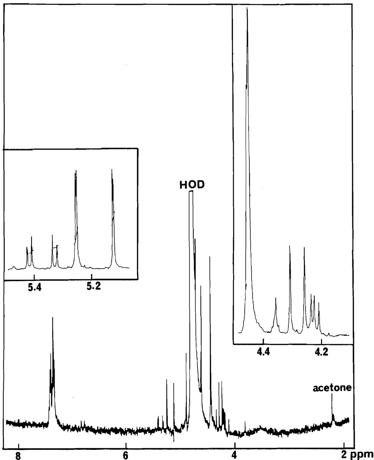
FIG. 2. The 400 MHz  $^1\text{H}$  NMR spectrum of benzimidazole after radiation chemical reduction in phosphate buffered  $\text{D}_2\text{O}$  at pH 7. This spectrum was obtained directly on the irradiated  $\text{D}_2\text{O}$  solution.
