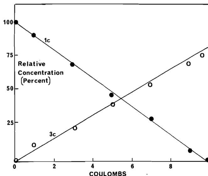
FIG. 4. Relative concentration of benznidazole **1c** and the product **3c** as a function of the number of coulombs passed through the solution in the electrochemical reduction of benznidazole. The initial concentration of benznidazole was 1.05 mM in a 25 mL volume (26.3  $\mu\text{mol}$ ). The relative concentrations of **1c** and **3c** were calculated from relative areas of the HPLC profiles, using standard curves constructed from injections of known amounts of authentic material.
