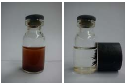
Figure 7. Separation of \gamma\text{-Fe}_2\text{O}_3\text{-2-HEAS} from the reaction mixture using an external magnet.
