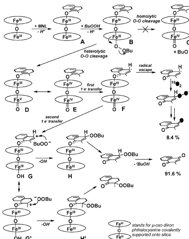
**Scheme 3** Proposed mechanism of oxidation of MNL by <sup>t</sup>BuOOH mediated by FePcS-SiO<sub>2</sub>.
