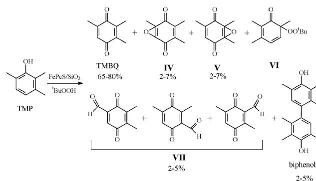
**Scheme 2** Oxidation of TMP by  $\text{tBuOOH}$  in the presence of FePcS- $\text{SiO}_2$ .
