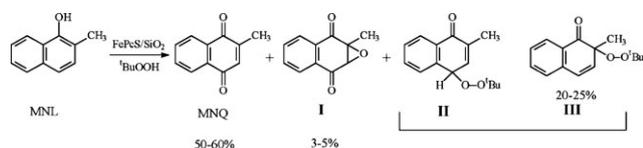
**Scheme 1** Oxidation of MNL by  $\text{tBuOOH}$  in the presence of FePcS- $\text{SiO}_2$ .
