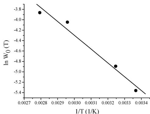
**Fig. 2** Temperature dependence of TMP oxidation with  $t$ BuOOH in the presence of FePcS-SiO<sub>2</sub>. Reaction conditions: [TMP] = 0.1 M, [ $t$ BuOOH] = 0.2 M, 3.2 mg of FePcS-SiO<sub>2</sub> (0.14 mol%), 1 mL of MeCN.
