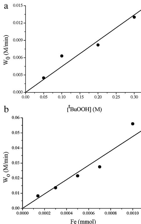
**Fig. 3** Dependence of the initial rate  $W_0$  on [ $t$ BuOOH] (a) and catalyst amount (b) in the TMP oxidation by  $t$ BuOOH mediated by FePcS-SiO<sub>2</sub>. Reaction conditions: [TMP] = 0.1 M, [ $\text{H}_2\text{O}$ ] = 0.65 M, 1 mL of MeCN, 35 °C; (a) 3.2 mg of FePcS-SiO<sub>2</sub> (0.14 mol% Fe); (b) [ $t$ BuOOH] = 0.2 M.
