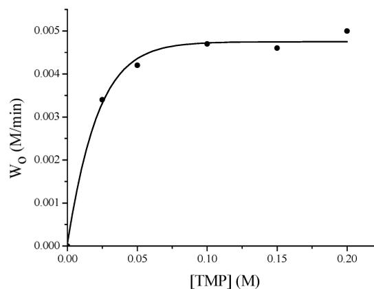
**Fig. 4** Dependence of the initial oxidation rate  $W_0$  on [TMP]. Reaction conditions: [ $t$ BuOOH] = 0.2 M, 3.2 mg of FePcS-SiO<sub>2</sub> (0.14 mol% Fe), [ $\text{H}_2\text{O}$ ] = 0.65 M, 1 mL of MeCN, 35 °C
