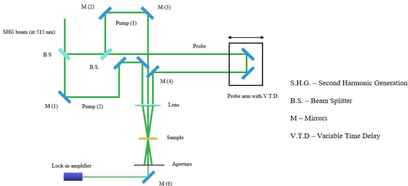
**Fig. 3** Experimental configuration of degenerate four-wave mixing using folded-box CARS geometry
