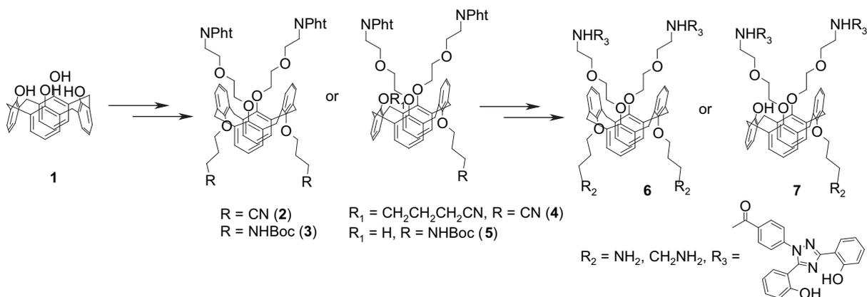
Fig. 2. Reactional sequence used to synthesize the key calixarenes as a preliminary step for the formation of the hybrid material.
