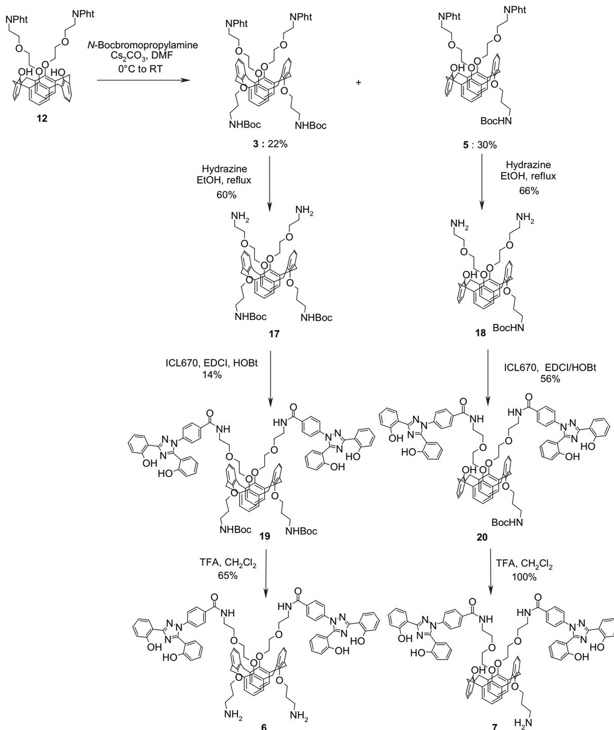
**Scheme 3.** Synthesis of the mono or diaminoalkyl diICL[4]arenes in 1,3-alternate **6** or in partial cone **7** conformation.
