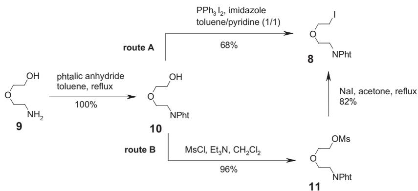
Scheme 1. Synthesis of the iodo arm spacer.
