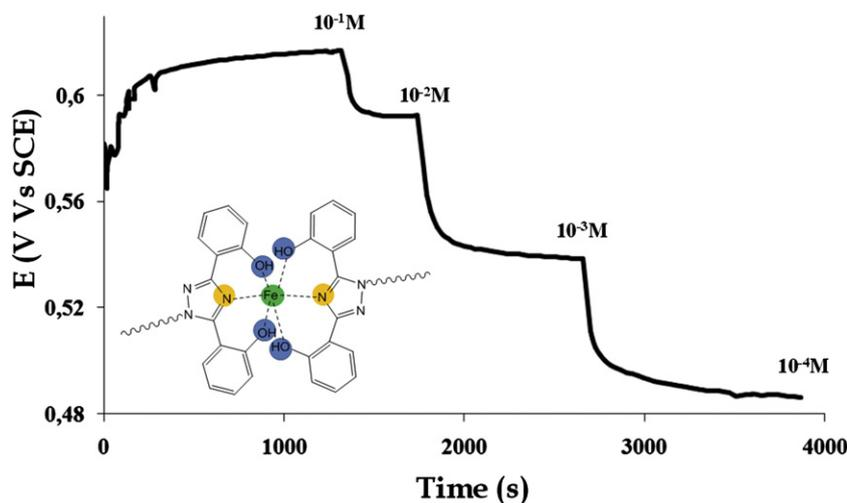
Fig. 4. Potentiometric response of the new electrode toward iron (III) aqueous solution over a range from  $10^{-1}$  mol/L to  $10^{-4}$  mol/L.
