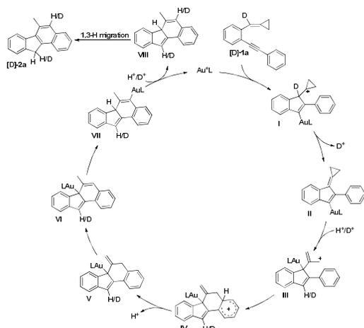
Scheme 5 A plausible reaction mechanism.
