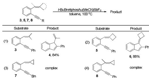
**Scheme 2** The supplementary experiment on the substrate scope
