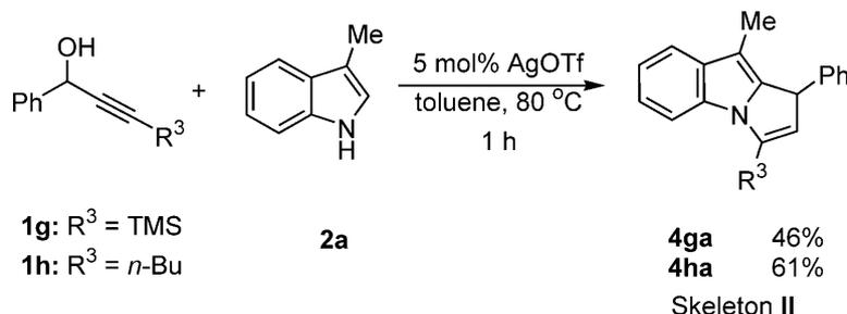
**Scheme 3.** Cascade reactions of TMS- and alkyl-substituted propargyl alcohols with 3-methyl-1*H*-indole.
