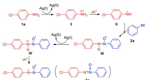
**Scheme 3.** Proposed reaction mechanisms.
