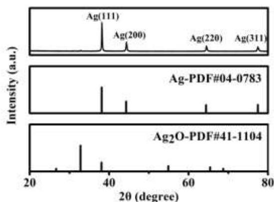
**Figure 2.** XRD diffraction patterns of the collected silver particles.
