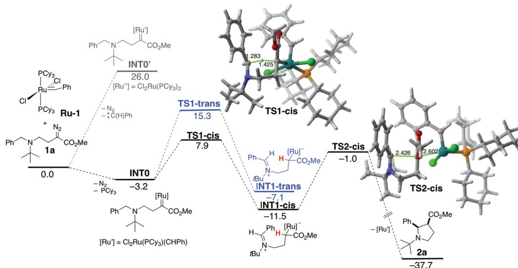
Fig. 2 Computed reaction profile for the formation of **2a** from **1a**. Relative free energies ( $\Delta G$ , at 298 K) and bond lengths are given in kcal mol<sup>-1</sup> and angstroms, respectively. All data have been computed at the PCM(CH<sub>2</sub>Cl<sub>2</sub>)-B3LYP-D3/def2-TZVPP//PCM(CH<sub>2</sub>Cl<sub>2</sub>)-B3LYP-D3/def2-SVP level.
