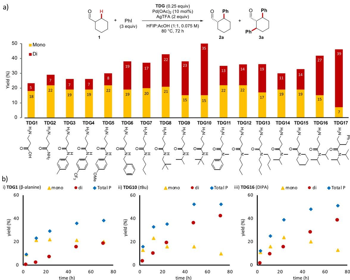
**Figure 1.** (a) Effect of amide transient directing groups on methylene C(sp<sup>3</sup>)-H arylation of cyclohexanecarboxaldehyde; results are averages of two runs. (b) Reaction profiles using (i)  $\beta$ -alanine, (ii) *t*Bu-amide TDG10, and (iii) DIPA-amide TDG16. Solvent system: HFIP/AcOH (5:1). Total P = yield of mono 2a + di 3a. Yields determined by <sup>1</sup>H NMR using 1,3,5-trimethoxybenzene as an internal standard.
