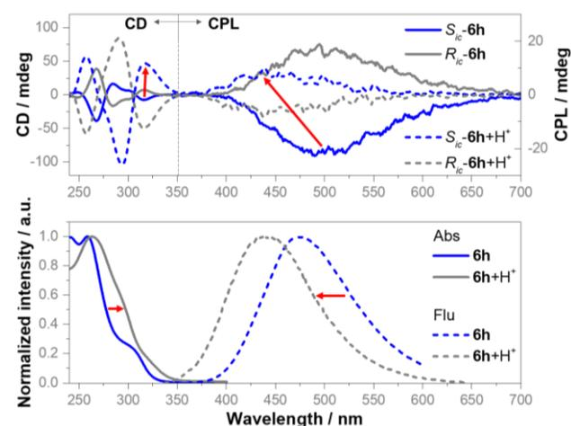
Figure 3. ECD (top left,  $2 \times 10^{-5}$  M), CPL (top right,  $1 \times 10^{-4}$  M,  $\lambda_{ex} = 310$  nm), UV/vis (bottom left,  $1 \times 10^{-5}$  M), and fluorescence (bottom right,  $1 \times 10^{-6}$  M,  $\lambda_{ex} = 310$  nm) spectra of (*S*<sub>ic</sub>)-**6h** and (*R*<sub>ic</sub>)-**6h**' in the absence and presence of CF<sub>3</sub>CO<sub>2</sub>H (10 equiv) in CH<sub>3</sub>CN.
