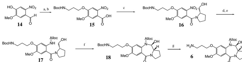
**Scheme 3.** Reagents and conditions: (a) PPh<sub>3</sub>, DEAD, (3-hydroxy-propyl)carbamic acid *tert*-butyl ester, THF; (b) KMnO<sub>4</sub>, water, acetone, 32% over 2 steps; (c) *S*-pyrrolidinemethanol, EDCI, HOBt, DMF, 93%; (d) 10% Pd/C, H<sub>2</sub>, EtOAc, quant; (e) allyl chloroformate, pyridine, DCM, 86%; (f) TEMPO, BAIB, DCM, 72%; (g) TFA, DCM, water (47/47/6), quant.
