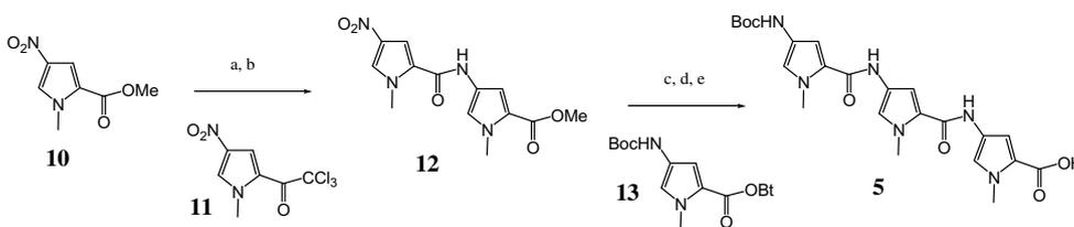
**Scheme 2.** Reagents and conditions: (a) 10% Pd/C, H<sub>2</sub>, DMF, quant; (b) **11**, DMF, 50%; (c) 10% Pd/C, H<sub>2</sub>, DMF, quant; (d) **13**, DMF, 94%; (e) NaOH, MeOH, water, quant.
