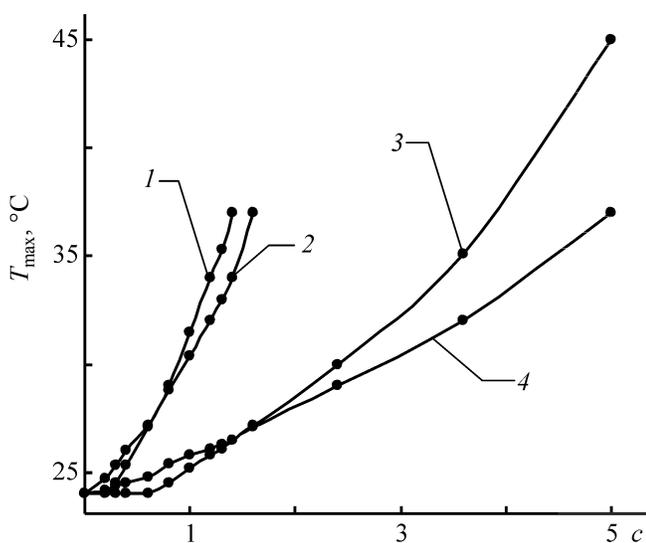
**Fig. 5.** Maximum temperature  $T_{\text{max}}$  of the reaction mass vs. the  $\text{TiO}_2$  content  $c$ . (1, 2)  $\text{TiO}_2\text{-PCe}$  and (3, 4)  $\text{TiO}_2$ . (1, 3) Reaction in the presence of TMP and (2, 4) without a substrate.
