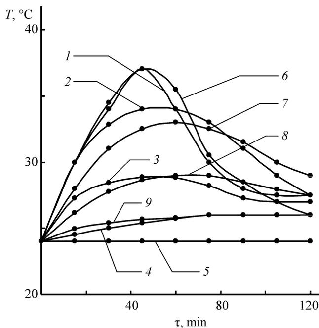
**Fig. 4.** Reaction mass temperature  $T$  vs. the reaction duration  $\tau$  on  $\text{TiO}_2\text{-PCe}$ .  $\text{H}_2\text{O}_2/\text{TiO}_2$  molar ratio: (1) 5.4, (2) 6.2, (3) 9.4, (4) 18.7, and (5) 31.2 (in the presence of the substrate); (6) 4.7, (7) 5.9, (8) 9.4, and (9) 18.7 (in the absence of a substrate).
