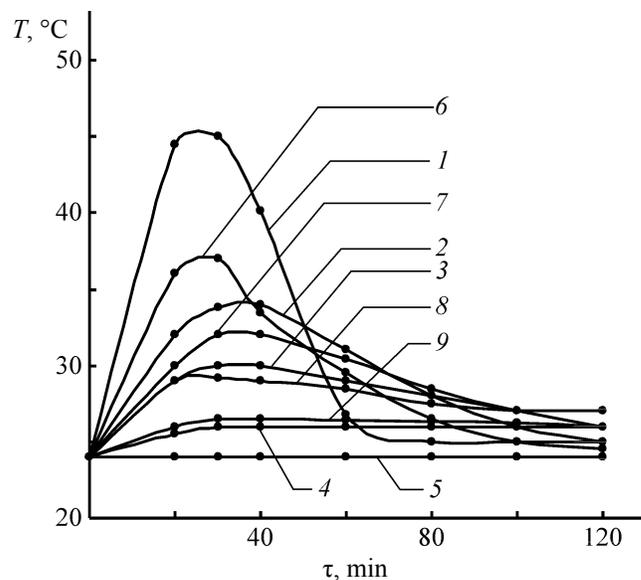
Fig. 3. Reaction mass temperature  $T$  vs. the reaction duration  $\tau$ .  $\text{H}_2\text{O}_2/\text{TiO}_2$  molar ratio: (1, 6) 1.5, (2, 7) 2.1, (3, 8) 3.1, (4, 9) 6.2, and (5) 12.5–25.0. (1–5) In the presence of the substrate, (6–9) in the absence of a substrate.
