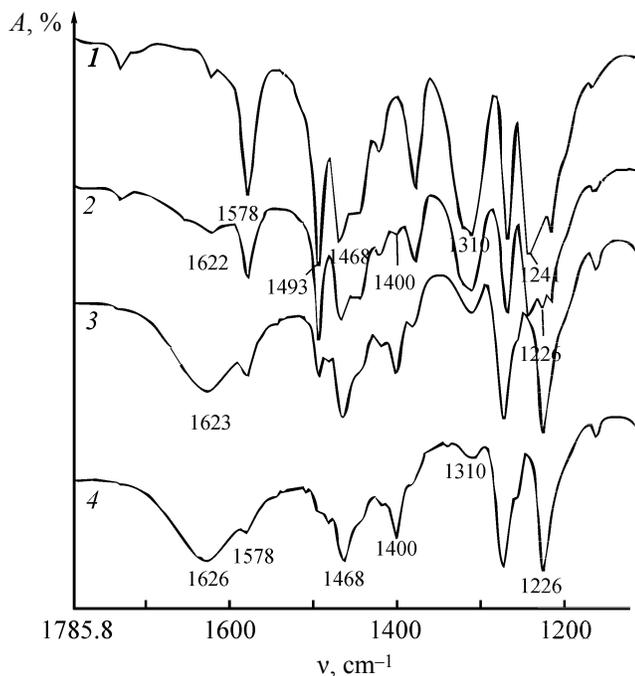
**Fig. 1.** IR spectra of TMP sorbed on the  $\text{TiO}_2$  xerogel. (A) Absorption and ( $\nu$ ) wave number. (1)  $\text{TiO}_2$ ;  $\text{TiO}_2$  : TMP mass ratio: (2) 1 : 2, (3) 1 : 1, and (4) 1 : 0.5.
