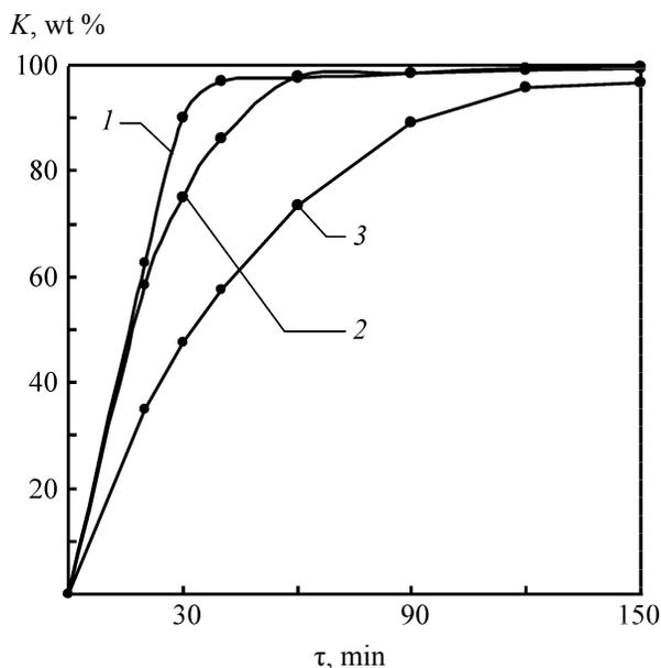
**Fig. 6.** TMP conversion  $K$  vs. the reaction duration  $\tau$ .  $\text{TiO}_2/\text{TMP}$  ratio: (1)  $\text{TiO}_2$  8.2–34.0, (2)  $\text{TiO}_2\text{-PCe}$  2.7, and (3)  $\text{TiO}_2\text{-PCe}$  1.6.
