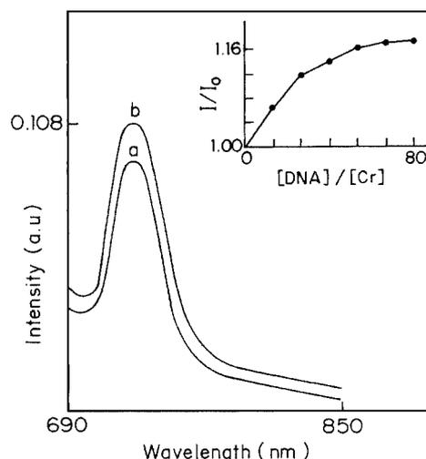
Figure 4. Emission spectra of  $[\text{Cr}(\text{bzimpy})_2]^+$  in aqueous solution in a) absence and b) presence of DNA.  $[\text{Cr}] = 10 \text{ mM}$ ,  $[\text{DNA}] = 200\text{--}800 \text{ mM}$ . Inset: Relative emission intensity of  $[\text{Cr}(\text{bzimpy})_2]^+$  versus  $[\text{DNA}]/[\text{Cr}]$
