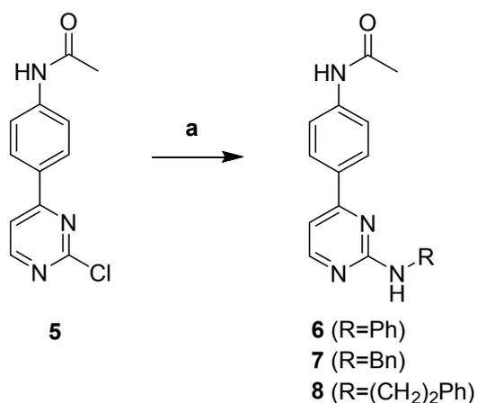
Reagents and Conditions: (a) aniline, benzylamine or phenethylamine, PTSA, nBuOH, 100°C, 2h.
