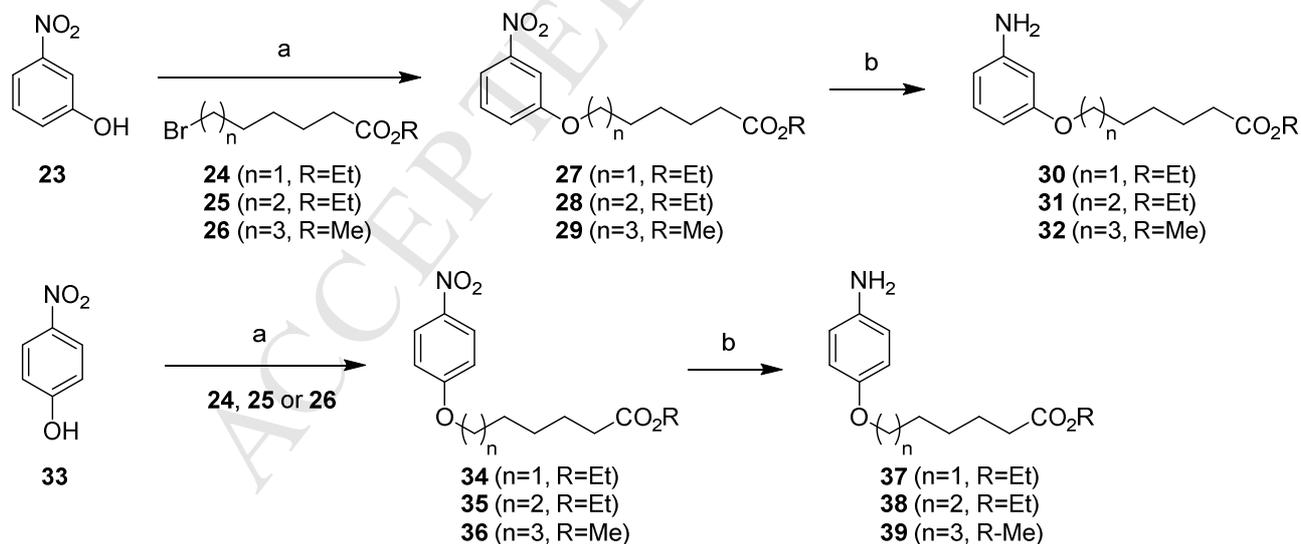
(a) K<sub>2</sub>CO<sub>3</sub>, MeCN, 80°C, 18h; (b) Fe, NH<sub>4</sub>Cl, MeOH/H<sub>2</sub>O (2:1), reflux, 3-18 h.
