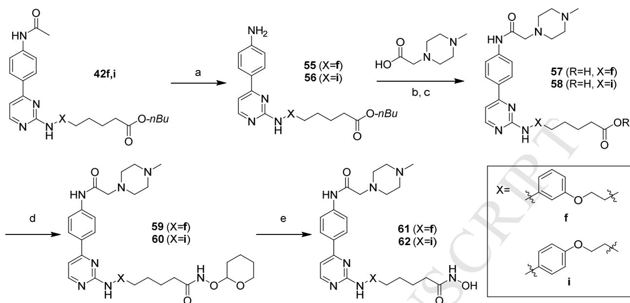
(a) 4N HCl/Dioxane, MeOH-THF, 50°C, 18h, 94%; (b) HATU, Et<sub>3</sub>N, THF, DMF, RT, 18h; (c) LiOH, THF/H<sub>2</sub>O (3:2), RT, 18h; (d) THPONH<sub>2</sub>, HATU, Et<sub>3</sub>N, DMF, RT, 18h; (e) AcCl, MeOH/DCM (1:10), RT, 3-18h
