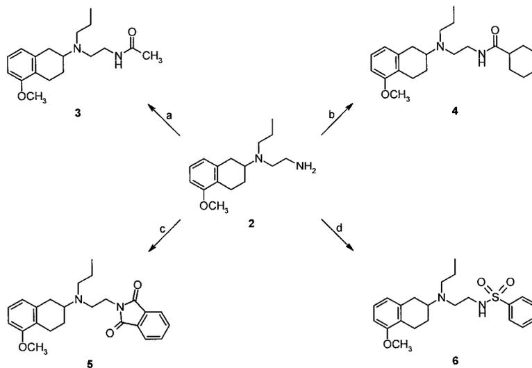
**Scheme 1.** Reagents and conditions: (a) Ac<sub>2</sub>O, NaOAc, EtOAc, H<sub>2</sub>O, rt; (b) C<sub>6</sub>H<sub>11</sub>COCl, 10% NaOH, CH<sub>2</sub>Cl<sub>2</sub>, rt; (c) phthalic anhydride, NaOAc, AcOH, Δ; (d) C<sub>6</sub>H<sub>5</sub>SO<sub>2</sub>Cl, K<sub>2</sub>CO<sub>3</sub>, CHCl<sub>3</sub>, H<sub>2</sub>O, rt.
