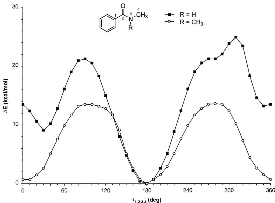
**Figure 1.** Rotation barriers around the amide bonds of *N*-methylbenzamide (R = H, black squares) and *N,N*-dimethylbenzamide (R = CH<sub>3</sub>, open circles), as obtained from AM1 calculations.
