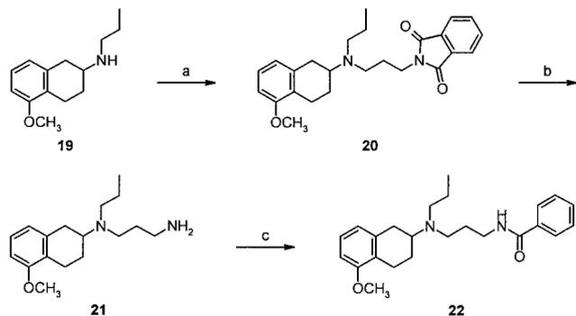
**Scheme 4.** Reagents and conditions: (a) *N*-(3-bromopropyl)phthalimide,  $\text{K}_2\text{CO}_3$ , KI, acetone,  $\Delta$ ; (b) hydrazine hydrate, EtOH, rt; (c)  $\text{C}_6\text{H}_5\text{COCl}$ , 10% NaOH,  $\text{CH}_2\text{Cl}_2$ , rt.
